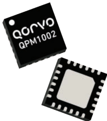
2. Qorvo's QPM1002 T/R FEM serves radar applications from 8.5 to 10.5 GHz. Qorvo
