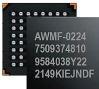
5. Anokiwave's AWMF-0224 IC integrates an LO synthesizer to translate between 24.25 to 29.50 GHz and IFs. Anokiwave
